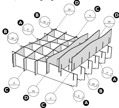
Loop ends of tension cord around tabs of outermost vertical sides. Repeat process for tension cord **(F)** as shown.
