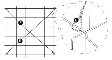
Twist ★ to tighten ♠. Loop tip of ★ around ♠ to hold in place.
