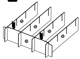
**Note**: To assemble correctly, align the slots perpendicularly to each other.
