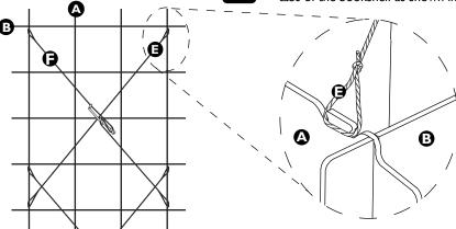
Twist X to tighten 🕒 . Loop tip of X around 🕞 to hold in place.
