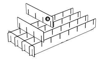
**Note**: To assemble correctly, align the slots perpendicularly to each other.
